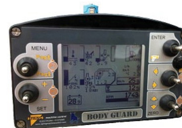
Engine data management via CAN J1939
