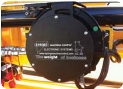
Cable reel with angular sensor and A2B management Management Over Drum Management End Rope
