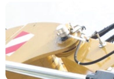
Option ZENITH sensor For a better precision of the arm movement limiter
