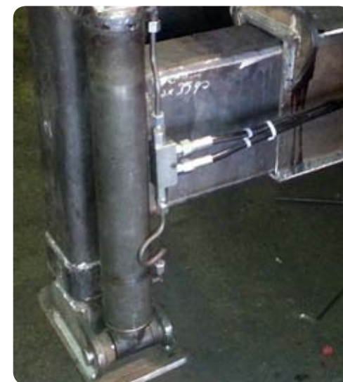
MANAGEMENT OF THE STABILIZER POSITION BY CABLE REEL SENSORS
