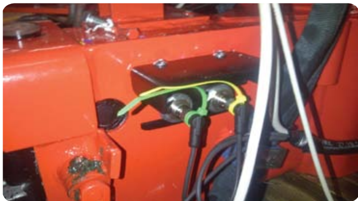
MANAGEMENT OF THE STABILIZER POSITION BY PROXIMITIES SENSORS
