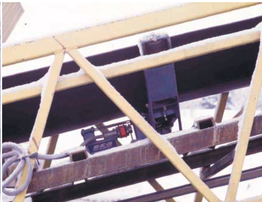
Weighing units can be installed in any ordinary conveyor with minimal disruption of operation.
