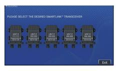
By utilizing a **Doran SmartLink™ One-Click™ Transceiver**. The tire pressure and temperature data on each vehicle is transferred from the transceiver to the SmartLink™ TPMS tablet, to instantly display data from all tires that are programmed to each piece of equipment.
