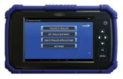
One-Click<sup>™</sup> Transceiver to quickly access and record digital tire pressure and temperature data from Individual Sensor Readings, Equipment Walk Arounds or by transferring the data from the SmartLink<sup>™</sup> One-Click<sup>™</sup> Transceiver.
